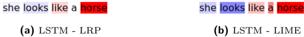
Figure 2: Heatmap visualization of the explanations made by LRP and LIME for a contextually toxic comment classified by an LSTM neural network.
